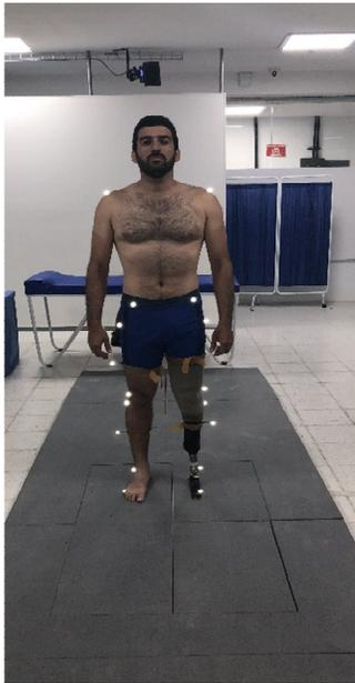
**Figure 7.** Retro reflecting markers attached to patient object of study.
