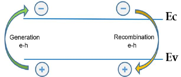
**Figure 10.** Sketch of a semiconductor in thermal equilibrium.  $E_v$  represents the valence band energy and  $E_c$  the conduction band energy, respectively. The electron-hole pair is denoted by  $e$ - $h$ . [18].
