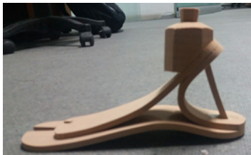
Figura 2. General assembly in micro porous sheets.
