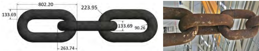
a. CAD model of test mooring chain with dimensions
