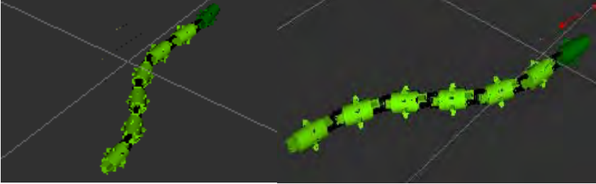
Figure 5: Result of robot simulation developing serpeneid curve in RVIZ-ROS.
