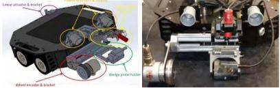
Figure 4. AWI's NDT payload.
