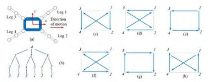
Figure 4: Sequence of quadruped walk
