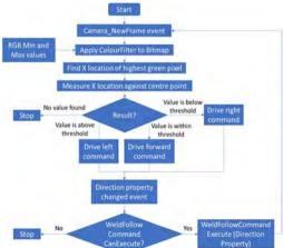
Figure 5. Weld following algorithm flow chart.
