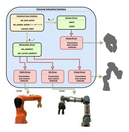
Fig. 1. Simplified UML class diagram of UII architecture.
