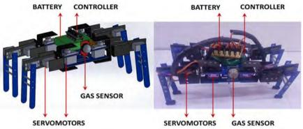
Figure 1: Quadruped robot design and prototype.
