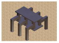
Fig. 1 3D CAD model of a 6-legged robot
