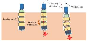
Figure 2. Overview of curved excavation.
