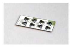
Fig. 3. A prototype of the thermomechanical walking platform [12]
