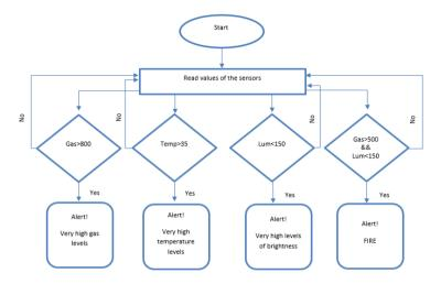
Figure 3- Flowchart of Operation
