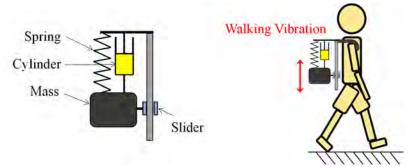
Figure 2. Operation of air compression device using walking vibration energy.
