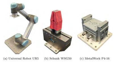
Fig. 4. Examples of robots and grippers adapted to fit the modular hardware concept.
