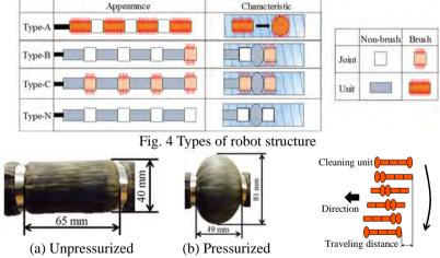
Fig. 5 Appearance of a driving unit
