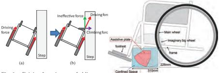
Fig. 1. Driving force in case of oblique approach to a step
