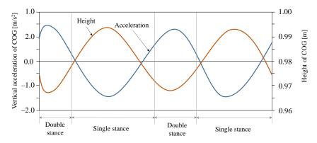
Figure 1. Height and acceleration of the center of gravity during a complete gait cycle.
