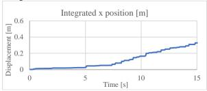
Figure 6. Position response on the physical SBP during experimental tests at 1Hz and  $45^{\circ}$  of amplitude in actuation
