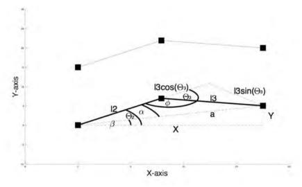
Figure 2: Mathematical & geometrical representation of joints 2 & 3
