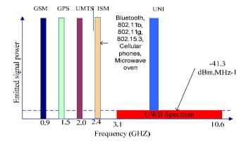
Figure 2. The different systems in ultra-high and super high frequency band.
