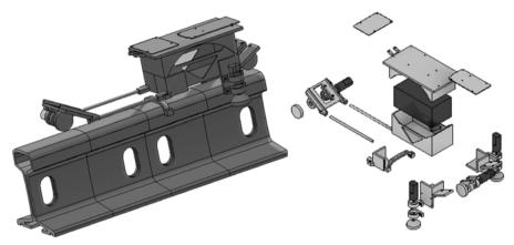
Figure 1a. Assembly of Robot and Track
