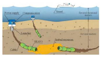
Figure 1. Concept of sub seafloor excavation robot(SEAVO).
