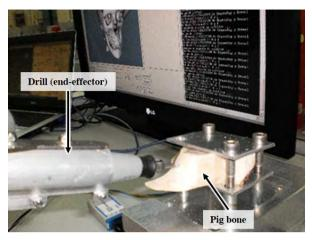
Figure 3. Final effector drilling a pig bone
