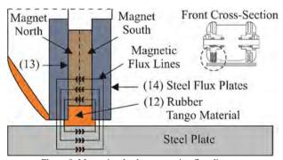
Figure 8: Magnetic wheel cross-section flux diagram.
