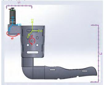
Figure 1: Design of shoulder rehabilitation robot first and second joint.
