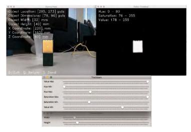
**Figure 6:** Visual recognition program detecting and localising object with respect to robot base.
