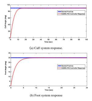
Figure 11. Calf and foot system response using HSDBC-PID controller.
