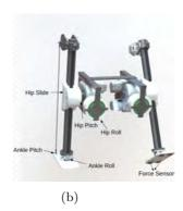
Fig. 1: An overview of SLIDER (a) Diagram of the SLIDER concept. (b) A rendering CAD model of SLIDER, showing all degrees of freedom
