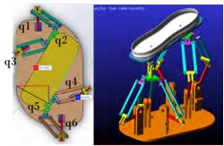
Figure 5. Kinematic analysis based on the position of the final effector generated by MSC Adams.
