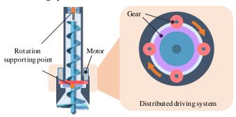
Figure 5. Concept of the distributed driving system.
