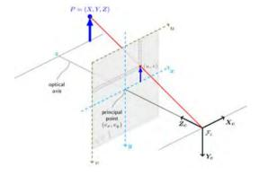
Figure 3: Pinhole camera model [10].
