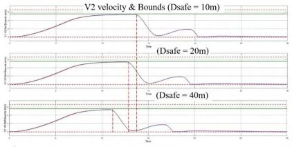
Figure 4. Speed curves at different safety distance values.
