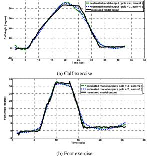
Figure 8. Measured and estimated model output for calf and foot
