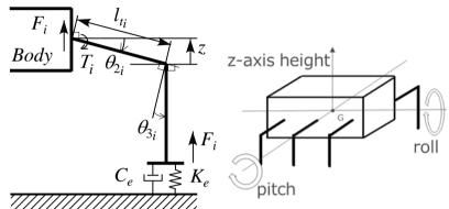
Fig.4 Relationship between the angle of thigh and the force in the perpendicular direction of the supporting leg
