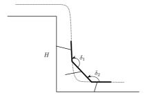
Fig. 3. Body inverse kinematics through simple linear approximation.
