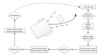
Fig. 6: Obstacle avoidance State Machine
