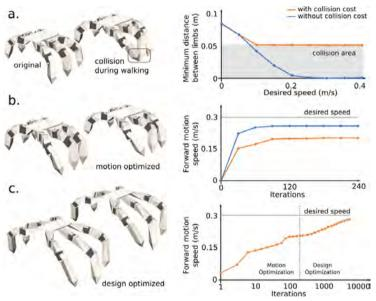
Figure 3. (a) Collision in a hexapod's limbs at high speeds. (b) Accounting for collisions in motion optimization prevents this, but also restricts the robot from walking faster. (c) Instead, design optimization increases spacing between limbs and their lengths.
