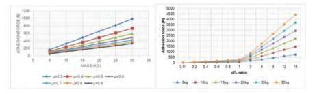
Figure 2. Minimum adhesion at different friction Figure 3. Effect of d/L on Adhesion force. coefficient, u.
