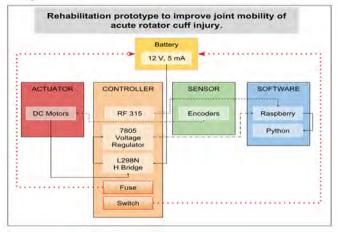
Figure 2: Schematic diagram of control architecture.
