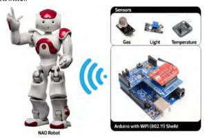
Figure 2- Architecture integrating three sensors to NAO robot
