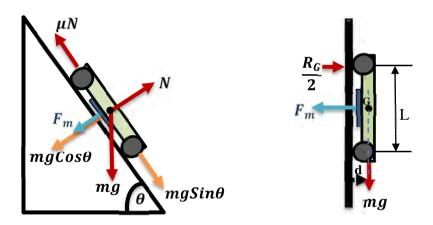
Figure 1. Robot on inclined surface.
