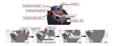
Fig. 5. Movement of the Lock function
