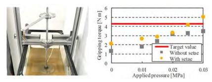
Figure 8. Measurement environment and result of gripping torque.
