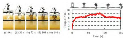
Figure 6. Excavation process and result of excavation torque.
