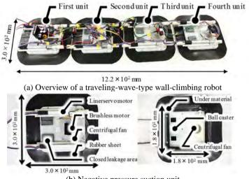
(b) Negative pressure suction unit Fig. 5 Traveling-wave-type wall-climbing robot
