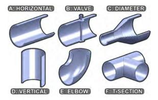
Figure 2: Common in-pipe obstacles A-F.
