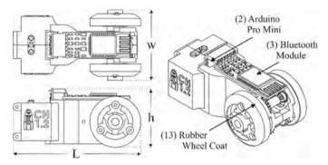
Figure 5: (a) Geometry of the magnetic robot.
