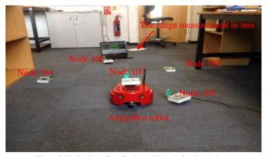
Figure 5. Mechanism of localization with the device descriptions.
