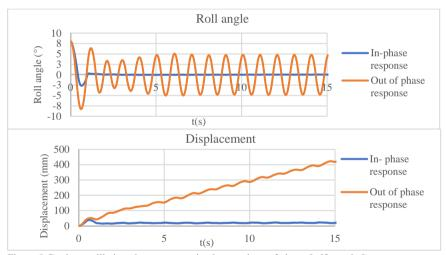
Figure 5. Rocker oscillation phase response in phase and out of phase (half a period).
