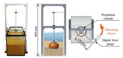
Figure 7. Experiment setup of propulsion unit.
