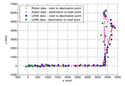
Figure 13. Test 4- positioning of the mobile robot using Odometry & orientation sensors and UWB from point A to B and from B to A.
