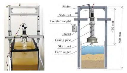
Figure 5. Experiment setup of excavation unit.
