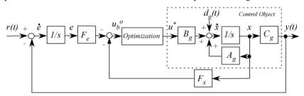
Fig.6 Block diagram of optimal servo with optimization
