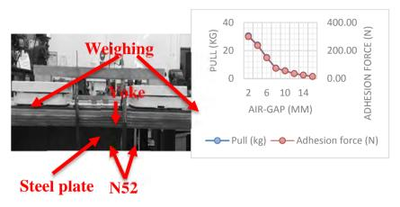
Figure 9. Experimental set-up.
