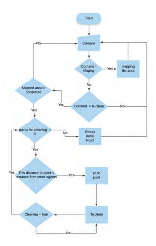
Figure 2. Control software flowchart
