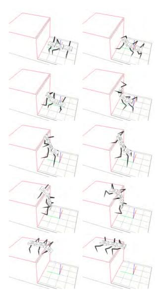
${\bf Fig.~7.} \quad {\bf Climbing~motion~sequence~(left-to-right,~top-to-bottom)}.$
