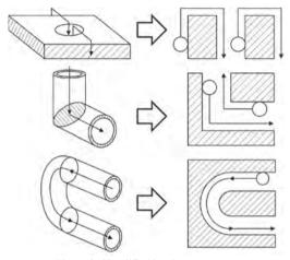
Figure 3: Simplified in-pipe geometry.
