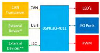
Figure 3: Block diagram of the electronic card.
