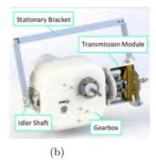
Fig. 2: (a) The inner view of the hip gearbox, it shows the transmission of vertical hip slide and hip pitch. (b) A side view of the gear motorbox and the hip roll transmission.
