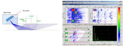
Figure 7. a) PA probe is mounted in the roller probe at 19°. b) Example of c-scan measured from the weld showing identification of defects.
