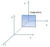
Figure 1. Pinhole Camera Model. Coordinates reference frames.
