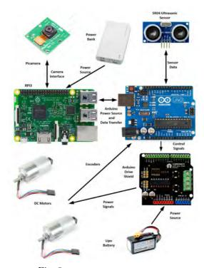
Fig. 3: Robot Prototype Components
