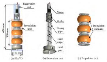
Figure 2. Overview of the excavation robot.
