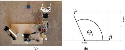
**Figure 1:** (a) Physical representation of ioint 1. (b) Mathematical representation of joint 1.
