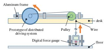
Figure 9. Overview of the power check experiment.
