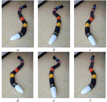
Figure 6: Motion sequence of the implemented robot like snake.
