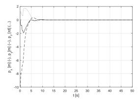
Fig. 2. Robot position and orientation errors (simulation results)
