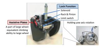
Fig. 3. Assistive Wheelchair Caster Unit (2nd prototype)
