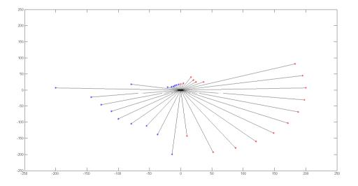
Figure 3. A  $360^{\circ}$  scan obtained from the fusion of the information from the three sensors (dimensions in cm.).
