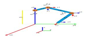
Figure 2. Kinematic model of the legs.
