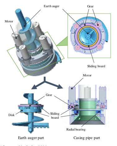
Figure 6. Prototype of the distributed driving system.
