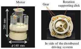
Figure 8. Appearance of the distributed driving system prototype.
